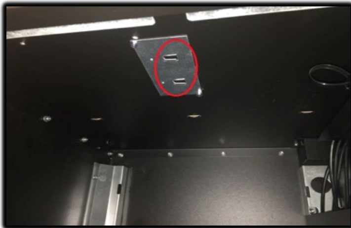
Control board mounting hooks
