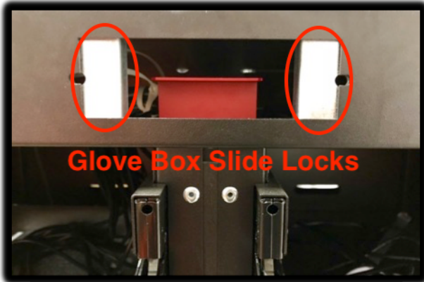
Locker door manual release lever in center and slide lock levers on each
